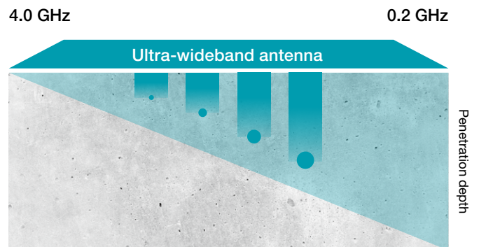
Proceq GPR Live covers all frequencies from 0.2 to 4.0 GHz with one single device. Lower frequencies allow deep penetration depths while higher frequencies allow for the detection of small objects.
