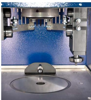
Compaction phase: simultaneous action of a static compression and of the shearing action
