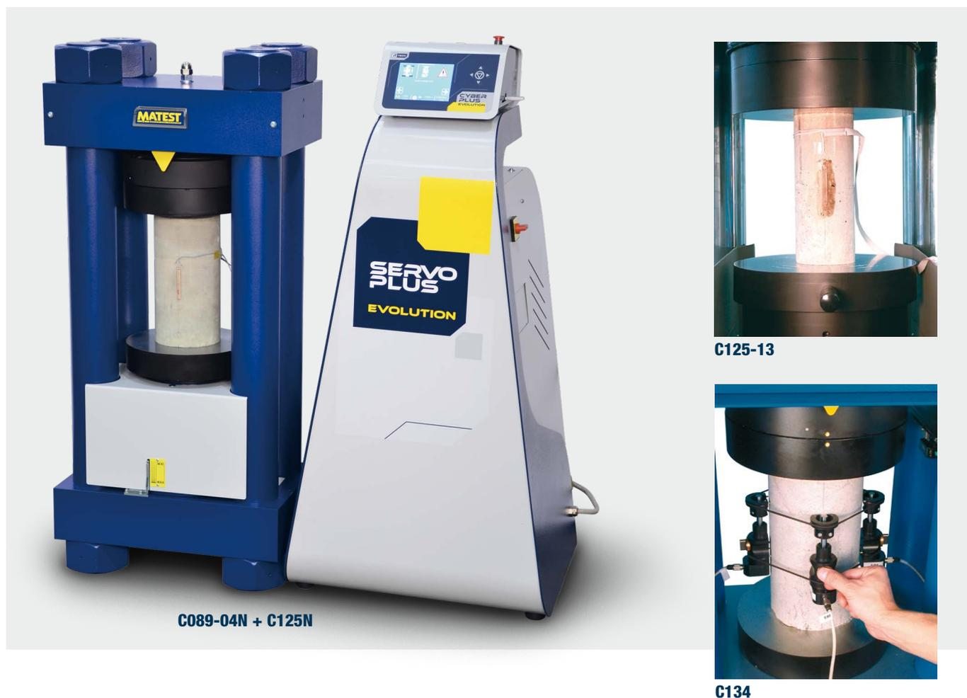
It can be used with a MATEST high stability frame 2000 or 3000 or 5000 kN capacity, coupled to the automatic servo-controlled system "Servo-Plus Evolution" (mod. C104N) housed in a separate pyramidal frame.
