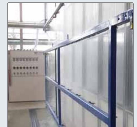
Spraying system for the watering according EN 12155.
