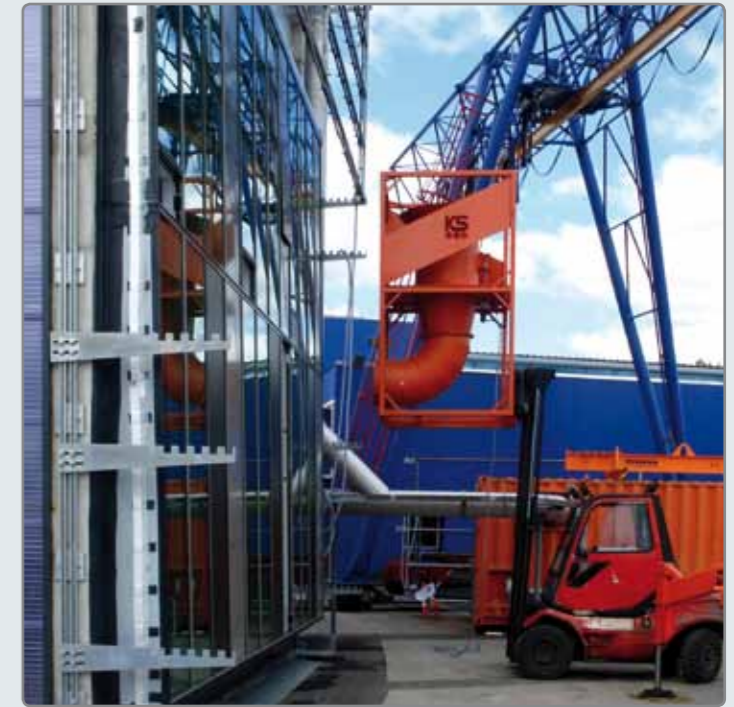
Wind generator* for the dynamic water tightness test according EN 13050.
