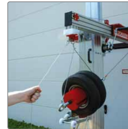
By pulling the ripcord the pendulum is released.
