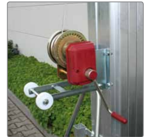
The mast is moved by a crank drive to the desired impact position.
