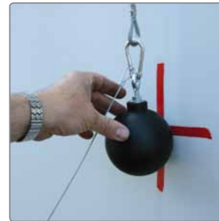
The bullet force the point of impact on the test block.
