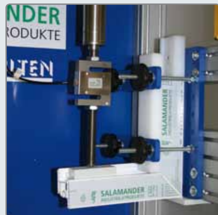
The Pull-Push unit is servo-controlled.
