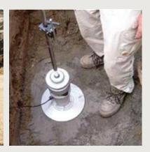
PRIMA 100 reads out your results at once. Results are stored automatically together with the GPS position. PRIMA100 applies wireless technology for data collection and is one-man operated
