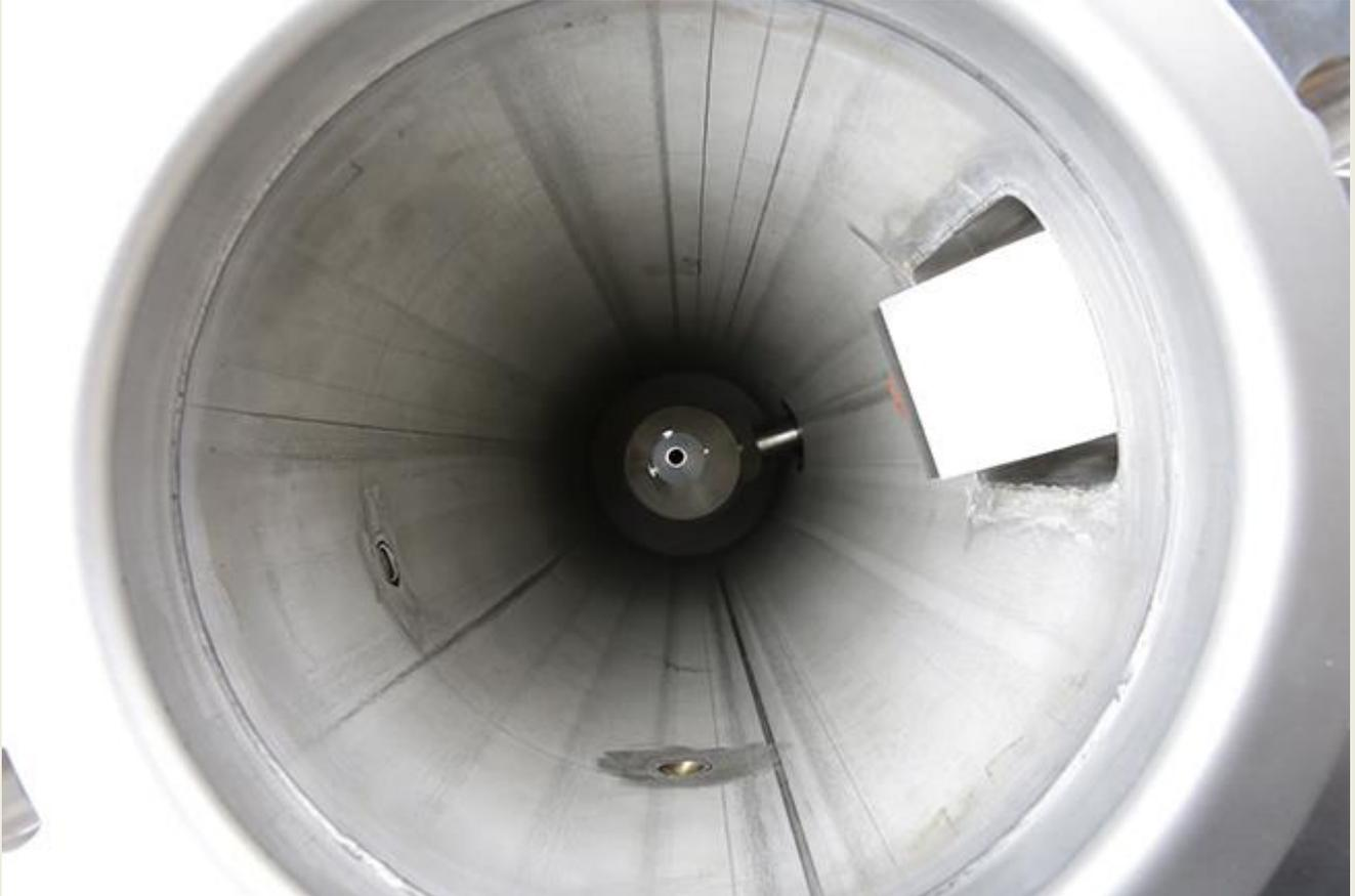
TWISTER 300+ for on-line measurement | Suitable for process lines from 300 mm (DN300) to over 800 mm (DN800) | ATEX version optionally available
