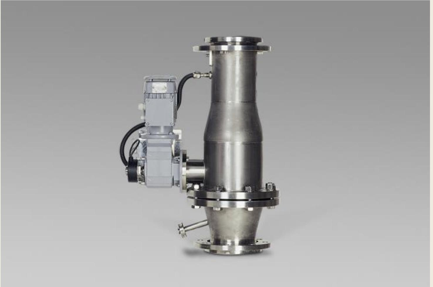
TWISTER 150 with expansion and attached reduction with sample ejector for on-line measurements | Suitable for process lines with a diameter of 150 mm (DN150) and for combination with in-line-MYTOS | ATEX and GMP versions optionally available
