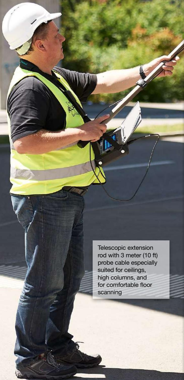
Telescopic extension rod with 3 meter (10 ft) probe cable especially suited for ceilings, high columns, and for comfortable floor scanning
