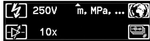
Rx gain, units, receiver gain, transmission mode
