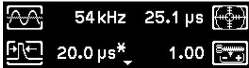
Tx frequency, calibration, pulse width, temperature correction
