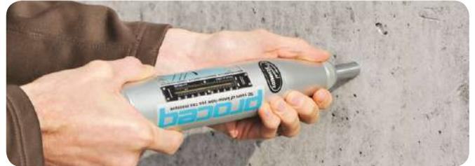
**Type N/L:** The benchmark against which all rebound hammers are compared and the basis of every international rebound hammer standard. Available with different impact energies allowing customers to test a wide variety of materials and types of structure.
